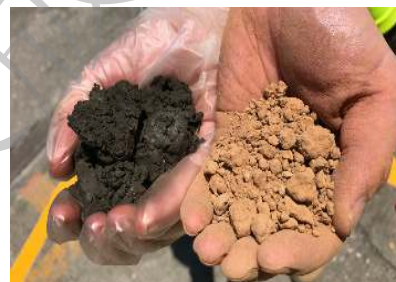
图7 T1 -3 实验阴燃反应前(左)、后(右)物料图 Fig. 7 Material of T1 -3 before and after smoldering
