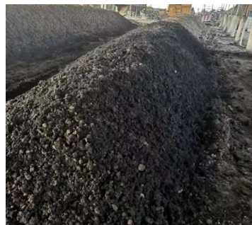
图1 餐厨垃圾衍生品条垛式堆肥现场 Fig. 1 Strip pile pilot test of food waste resource derivatives composting
